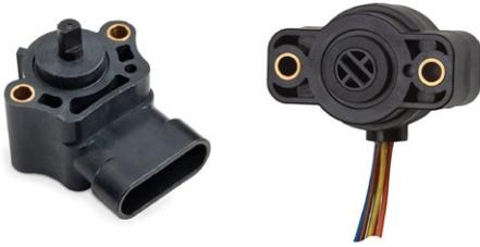
Hall effect sensors like Sensata's 9360 and 9960 models feature a standard operational life of 35 million cycles, linearity of +/-0.5%, up to IP69K sealing ratings and operating temperatures of 85° C; making them ideal for a wide variety of applications including fork inclination and steering control.
