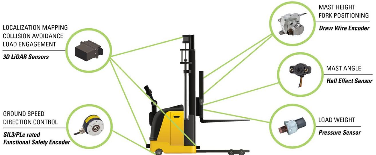
Hall effect sensors like Sensata's 9360 and 9960 models feature a standard operational life of 35 million cycles, linearity of +/-0.5%, up to IP69K sealing ratings and operating temperatures of 85° C; making them ideal for a wide variety of applications including fork inclination and steering control.
